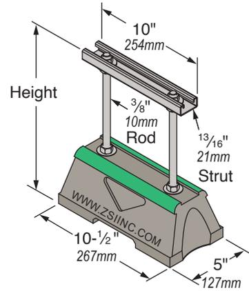
CBN-EX Extension Series Support with 3/8" Threaded Rod Extension and Pre-Galv. or Hot Dip Galv. Steel Channel
