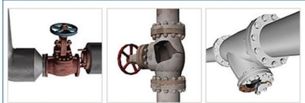
Water hammer problems can create extensive pipe damage. The magnetic shock detection device is a great tool to help maintenance crews detect water hammer areas BEFORE pipe damage occurs.
