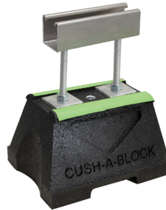
CBM-Support Extension with 3/8" Threaded Rod Extension & 1-5/8" (41mm) Pre-Galv or Hot Dip Galv. Steel Channel
